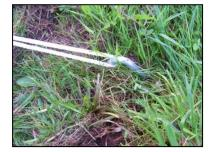
4.7.6 The tripod can also be anchored in the ground with the supplied stakes.
