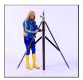
4.6.4 The telescopic mast in the centre may not touch the floor. Adjust the telescopic mast such that it is at least 10 cm above the floor.
