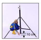
4.6.5 Adjust the cross braces so that they are parallel to the floor
